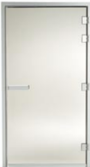
Steam Door 99 G (Art. 9091 2020) As above, but specially adapted for wheelchair access with extra wide opening and flat threshold. Frame dimensions: 1870 x 990 x 60 mm. Width of opening 880 mm.
