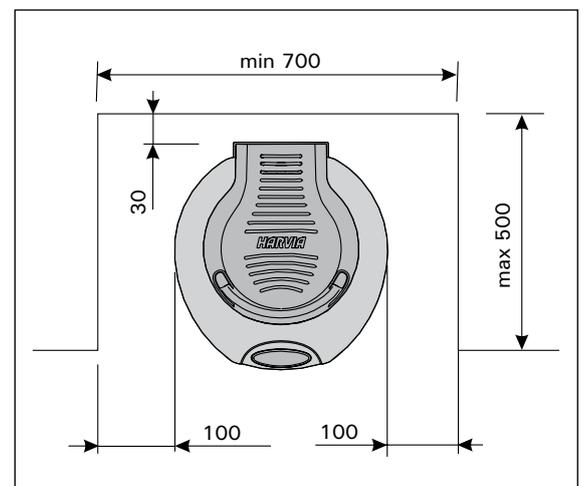
Figure 9. Installation of the heater in a recess
