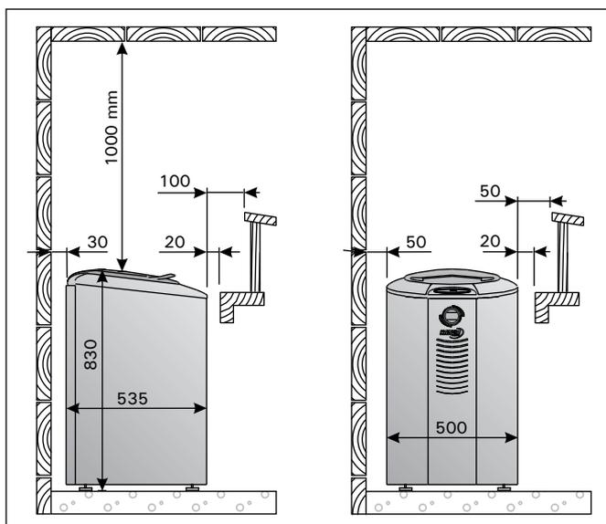
Figure 8. Minimum safety distances from the heater (mm)
