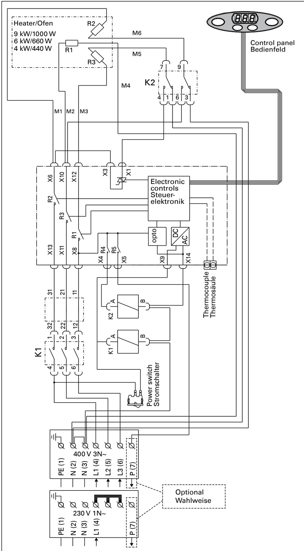
Figure 11. Electrical connections of heater
