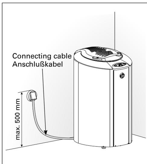
Figure 10. Connections of the heater
