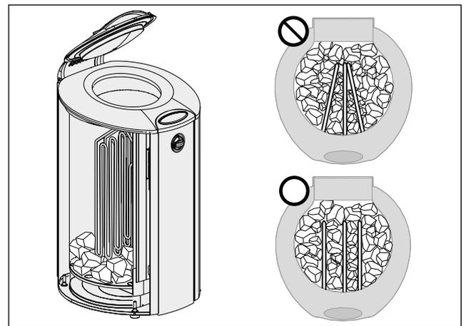
Figure 5. Supporting the heating elements.
