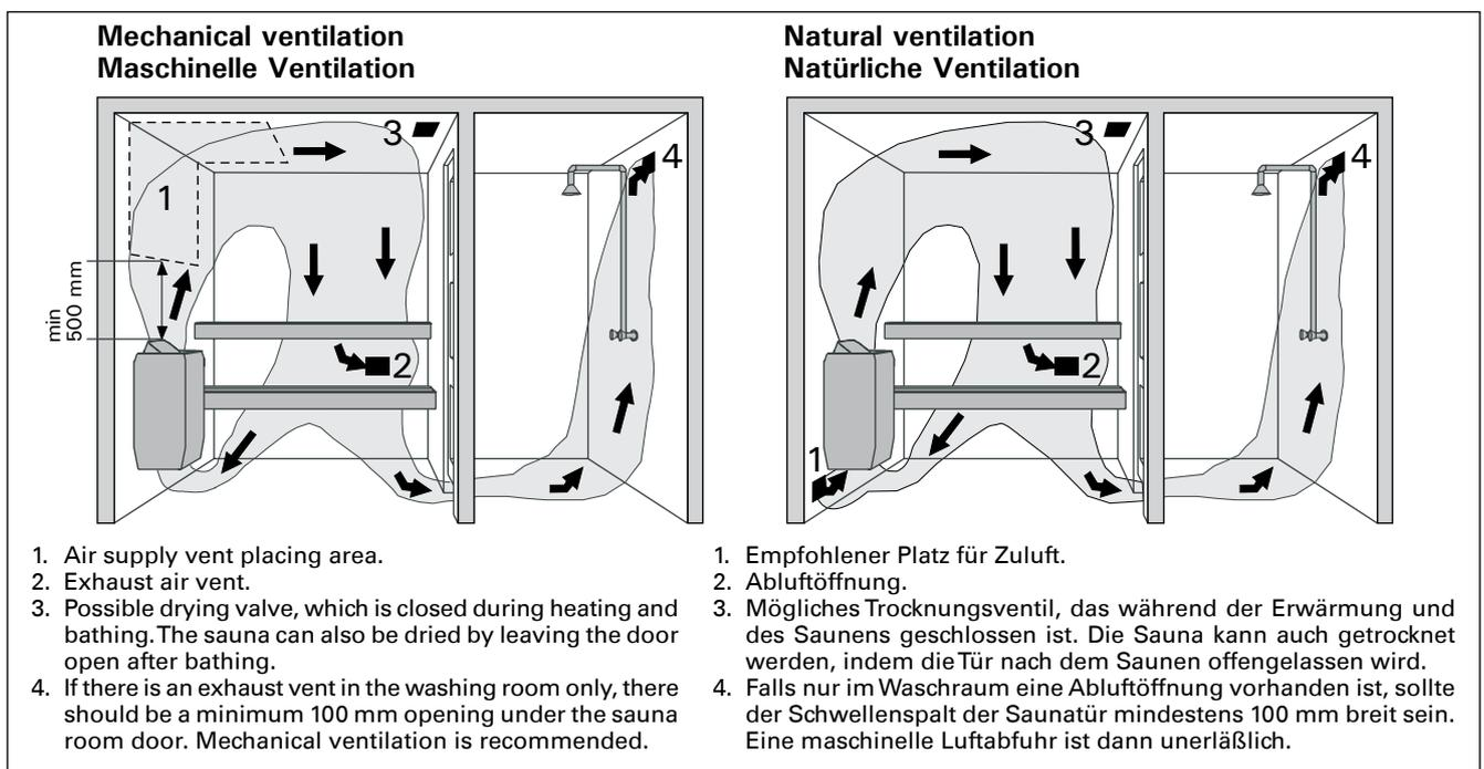
Figure 7. Ventilation of the sauna room
