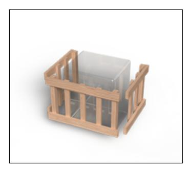
Some sauna heaters do not require a heater guard or fence, but if you were provided one in your kit, be sure to leave at least 2" of space between the heater and the guard, on all three sides. Assemble the heater guard before installing it in the sauna, using 15/8" screws to screw the front piece to the side pieces. Attach the side pieces to the walls using the same 15/8" screws. Install your vent covers over your vent openings, if provided with your kit.
