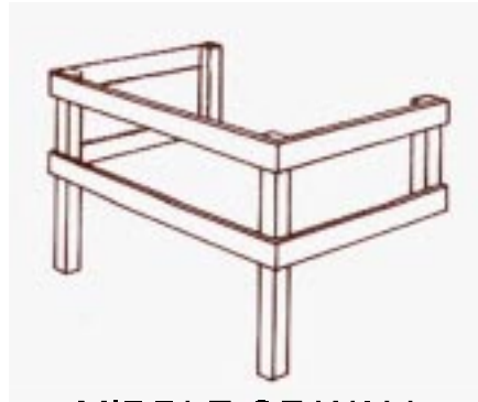
MIDDLE OF WALL HEATER GUARD
